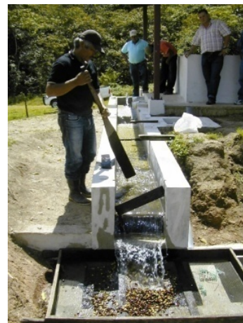
Ecologically friendly wet processing unit promoted by the CFC/ICO projects in Central America
