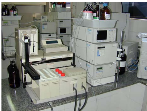
Figure 2: View of ASPEC-XL sample automatic processor and Shimadzu liquid chromatograph used for clean-up, separation, detection and quantification of OTA in green coffee.
