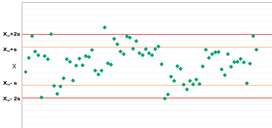
Figure 25: Example of Control chart of in-house material [naturally contaminated coffee sample, (4.99 + 0.58 \mu\text{g}/\text{kg} , n=20), n=78], SOP 039 ed. 03, rev. 02 (Immunoaffinity column clean-up and HPLC)
