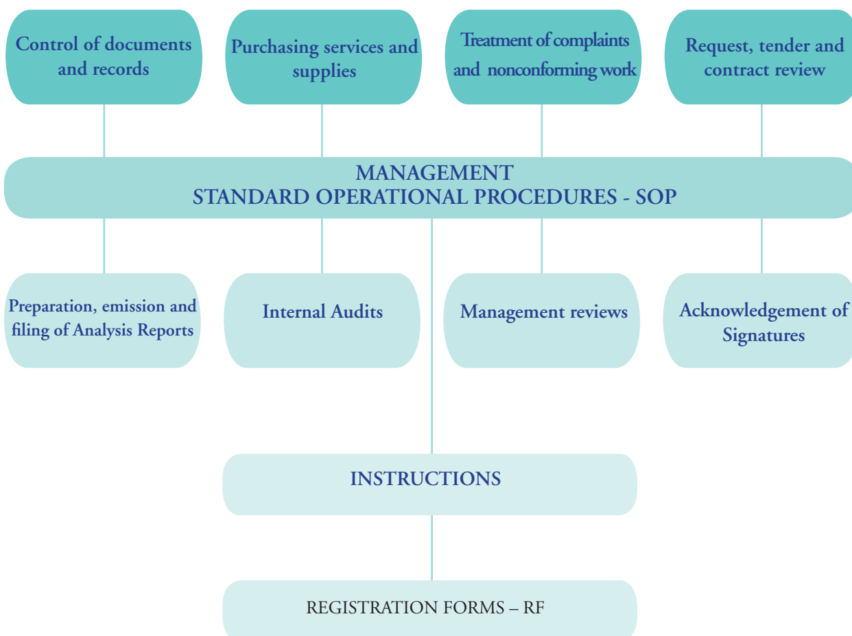
Figure 4: Example of principal documents established at LACQSA for compliance with management requirements – ISO 17025
