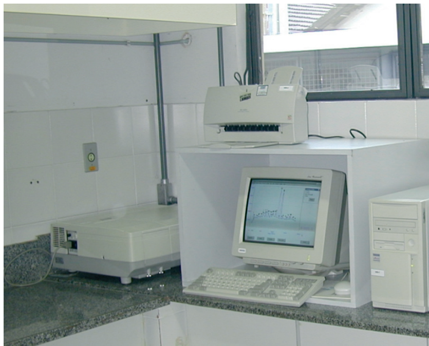
Figure 2: Spectrophotometer used for determination of OTA standard solution concentration
