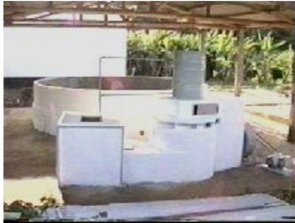
Fig. 10: General view of a fixed bed dryer (model designed at the Federal University of Viçosa, Brazil).
