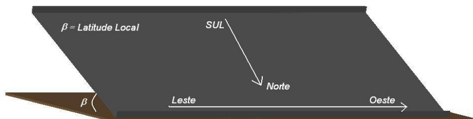
Fig. 6: Ideal fixed inclination for the solar energy 'roof collector' - about 20° latitude.
