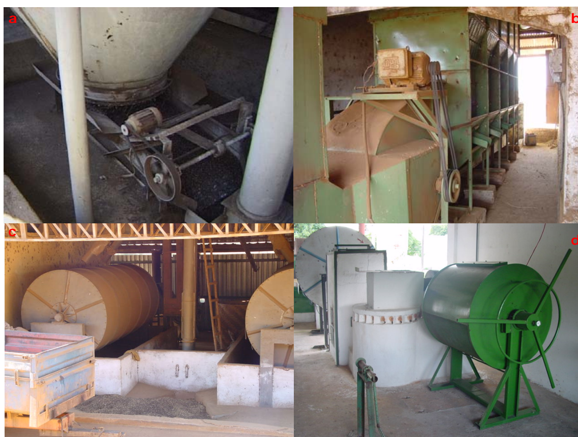
Fig. 12: a. Outlet funnel of vertical dryer; b. Drying chambers of vertical dryer; c. Horizontal dryer with continuous rotation of coffee; d. Prototype horizontal dryer developed by University of Viçosa, Brazil.
