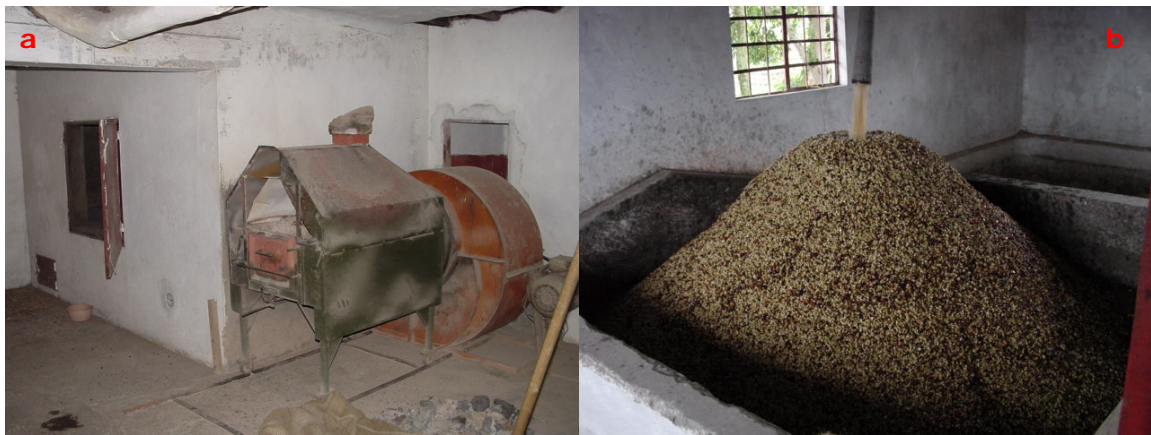
Fig. 9: a. Silo dryer; b. Pre-drying of wet parchment on the roof of a silo dryer
